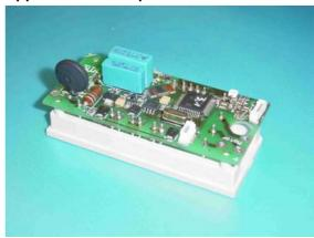
Shown is a complete frequency converter including the Gate Driver Circuit, the current sensing and the logic Power Supply and the Micro Controller with a interface for remote control. The power module used for this application is the Vincotech *flowPIM* 1
