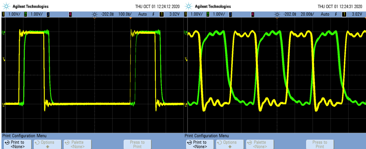
Figure 9 The delay between ClKI and the received ClKO on the control card on 1,6 MHz and 16 MHz
