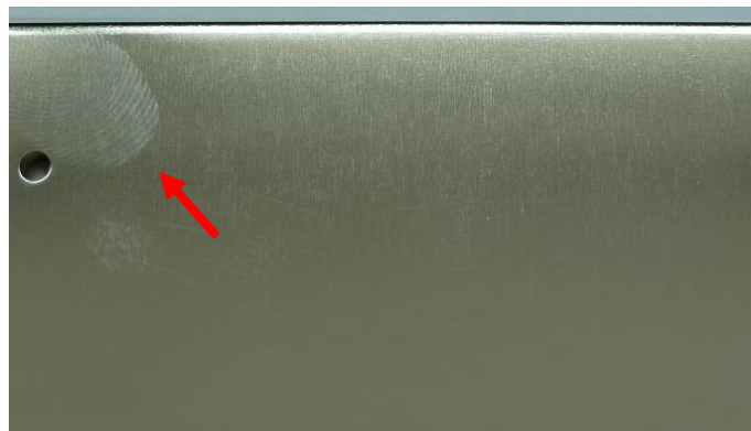
Figure 13: Fingerprint on the baseplate
