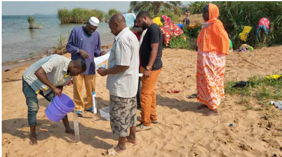
Fig. 3 Citizen scientists in Ujiji village measuring turbidity using turbidity tube (left)
