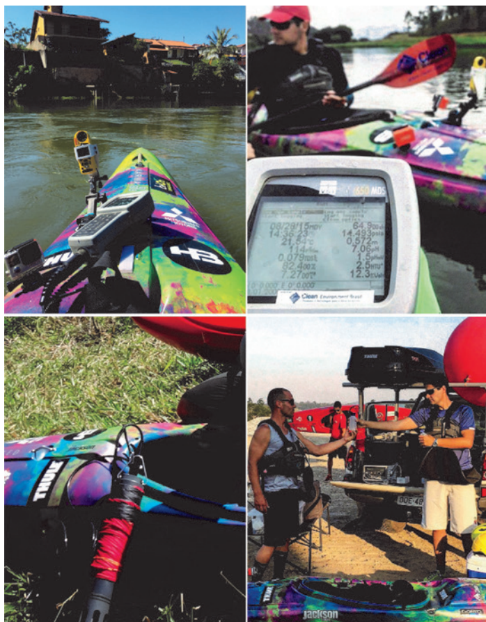
Figure 3: The professional kayak (Karma Unlimited Jackson Kayak) was adapted to be a data-sampling platform. Water quality probes, weather balloon, weather station, GPS and cameras collected data from the water, atmosphere and riverbanks. Photos by F. S. Pacheco and Pedro Oliva.
