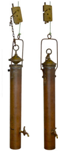
Fig. 4. Baldi's bottle , open (left) and closed (right). First half of the last century.
