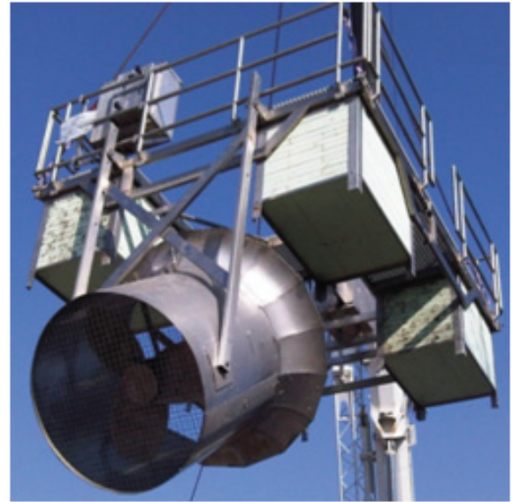
Figure 1 Propeller 1 – diameter 1.3m, speed 110 rpm
