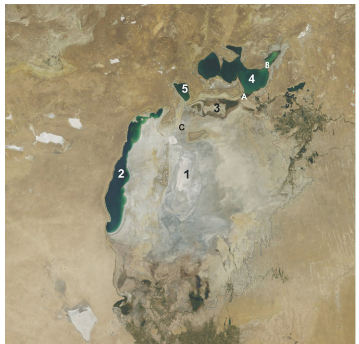
Fig.2. MODIS image of the Aral Sea acquired on August 19, 2014 (250 meter resolution; true color using bands 1-4-3): (1) dried Eastern Basin of the Large Aral Sea, (2) Western Basin of the Large Aral Sea, (3) New Central Aral Sea, (4) Small Aral Sea, (5) Tsche-Bas Bay. (A) Kokaral dam (Central dam), (B) Northern dam, (C) Southern dam. The faint line shows the 1960 dimensions of the Aral Sea. Source: NASA Earth Observatory ( http://earthobservatory.nasa.gov/IOTD/view.php?id=84437 ).
