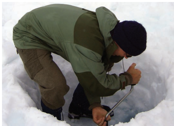
Lake Flakavatn at 1453 m.a.s.l., north of Finse, Norway. A 3-m drill may be needed to pierce a hole through the ice to access water - the hardest part of the sampling job (Photo: Trine Holm).
